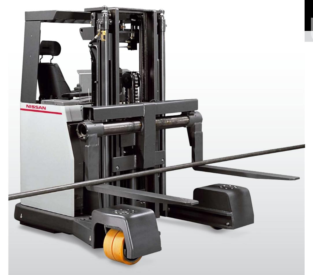
Four-way action allows the Nissan UFS reach truck to be operated in any direction with absolute precision. Typical use includes loading and unloading from ground level, internal transfer, and the stacking of normal, wide or long loads up to 9700 mm.
