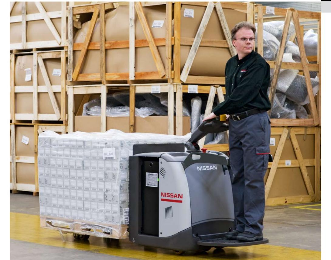
Stand-on, low-lift pallet transporter for medium to long distance travel, loading and unloading transport using dock levellers and occasional low level order picking. Robust chassis construction for medium to high intensity operations.
