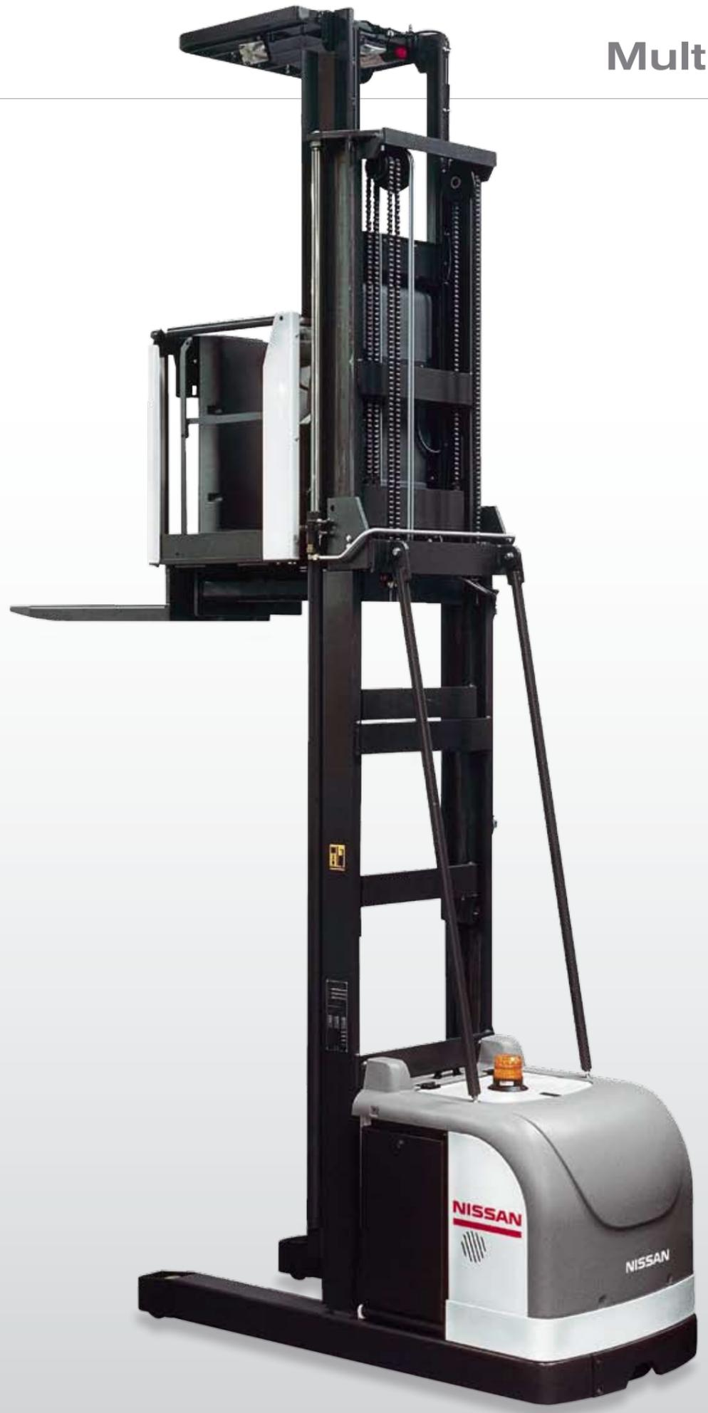
Nissan's range of high and multi-level order pickers extends to lift height of nearly 10 metres. Mast and chassis design together with a wide wheelbase offers exceptional stability and safety for operating at these extreme picking heights.
